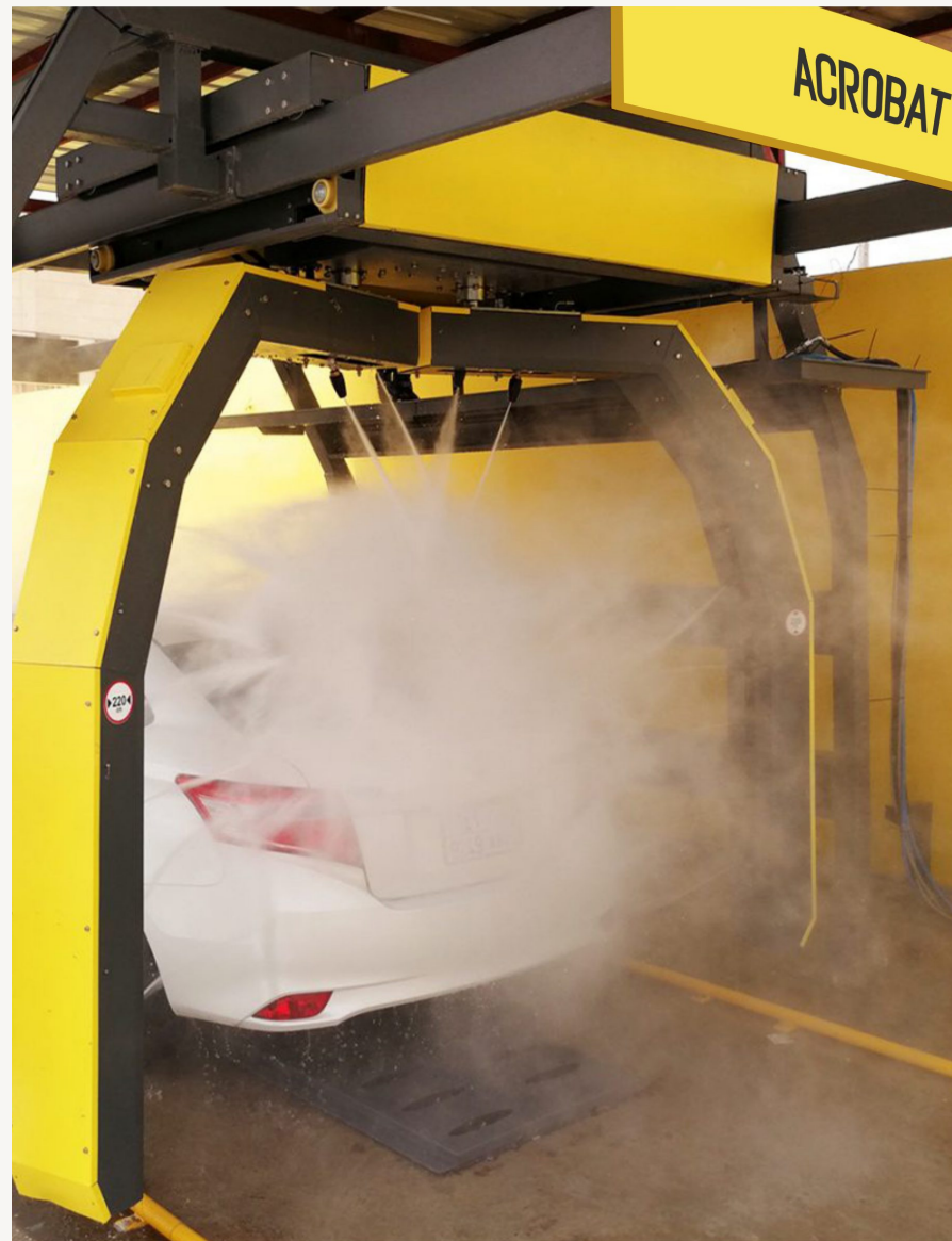
Acrobat 2X in service. Wash by water pressure and foam only, with the 220 cm width limit marked on the gantry leg.
