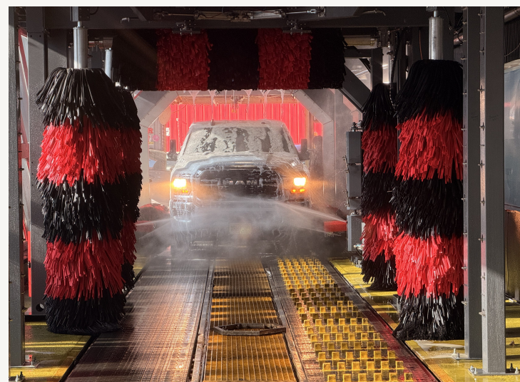
Power brushing. Two side brushes and a top brush work a vehicle as the conveyor carries it through.
