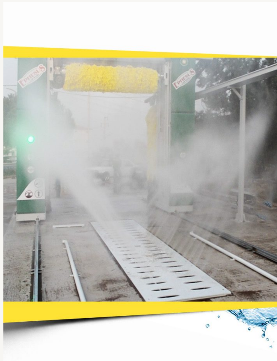
Ephesus in service. The machine runs on the rails set into the bay floor, with the drainage channel between them.
