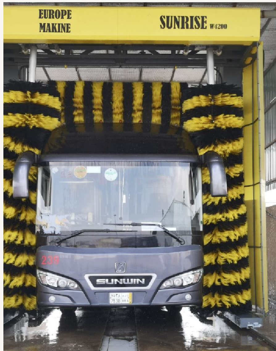
A SUNRISE gantry washing a bus. Two vertical brushes work the sides, one horizontal brush works the roof and the front. The machine photographed is a SUNRISE W4200.
